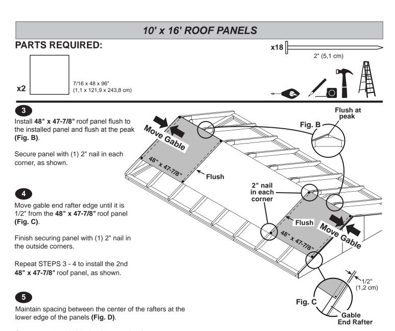
Secure panels with (1) 2" nail into each rafter, as shown.
