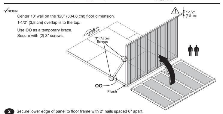
Secure wall bottom plates to floor with 3" nails (Fig. A).
