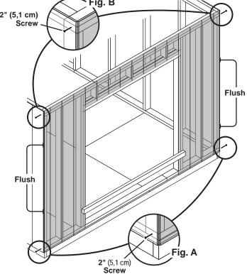
Nail lower edge of panels to floor with 2" nails spaced 6" apart. Angle nails into floor frame (Fig. C). Nail panels to 10' wall studs with 1-1/2"
