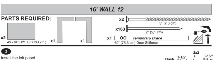
Flush (8,9 cm) (3.8 cm)1-1/2" from the top plate. BEGIN HERE (1,9 cm) Use a 2x3 spacer for consistent measurement. Secure panel with 2" **6"** (15,2 cm) nails spaced 6" apart on edges. -Flush Flush Install the right panel 3/4" Gauge flush to installed panel, Block as shown. (162,6 cm) Ensure 64" (162,8 cm) 00 Temporary Brace door measurement.
