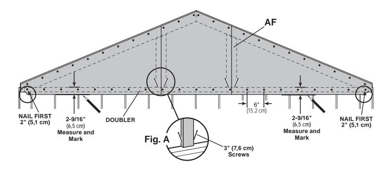
4 Continue securing panels to rafter with 2" nails spaced 6" apart.
