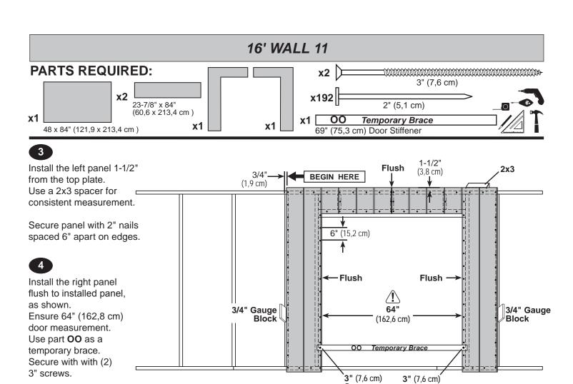
Secure panel with 2" nails spaced 6" apart on edges.
