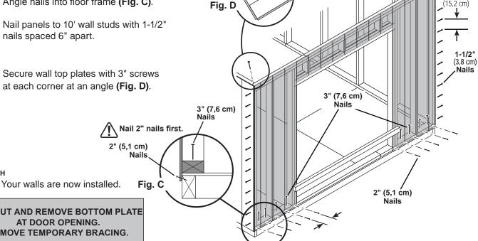
**CUT OUT AND REMOVE BOTTOM PLATE** AT DOOR OPENING. REMOVE TEMPORARY BRACING.
