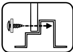
Always attach Wall Panels to Floor Frames with Screws as shown. Rest Panel on Floor Frame, aligning holes in the Panel and Floor Frame.
