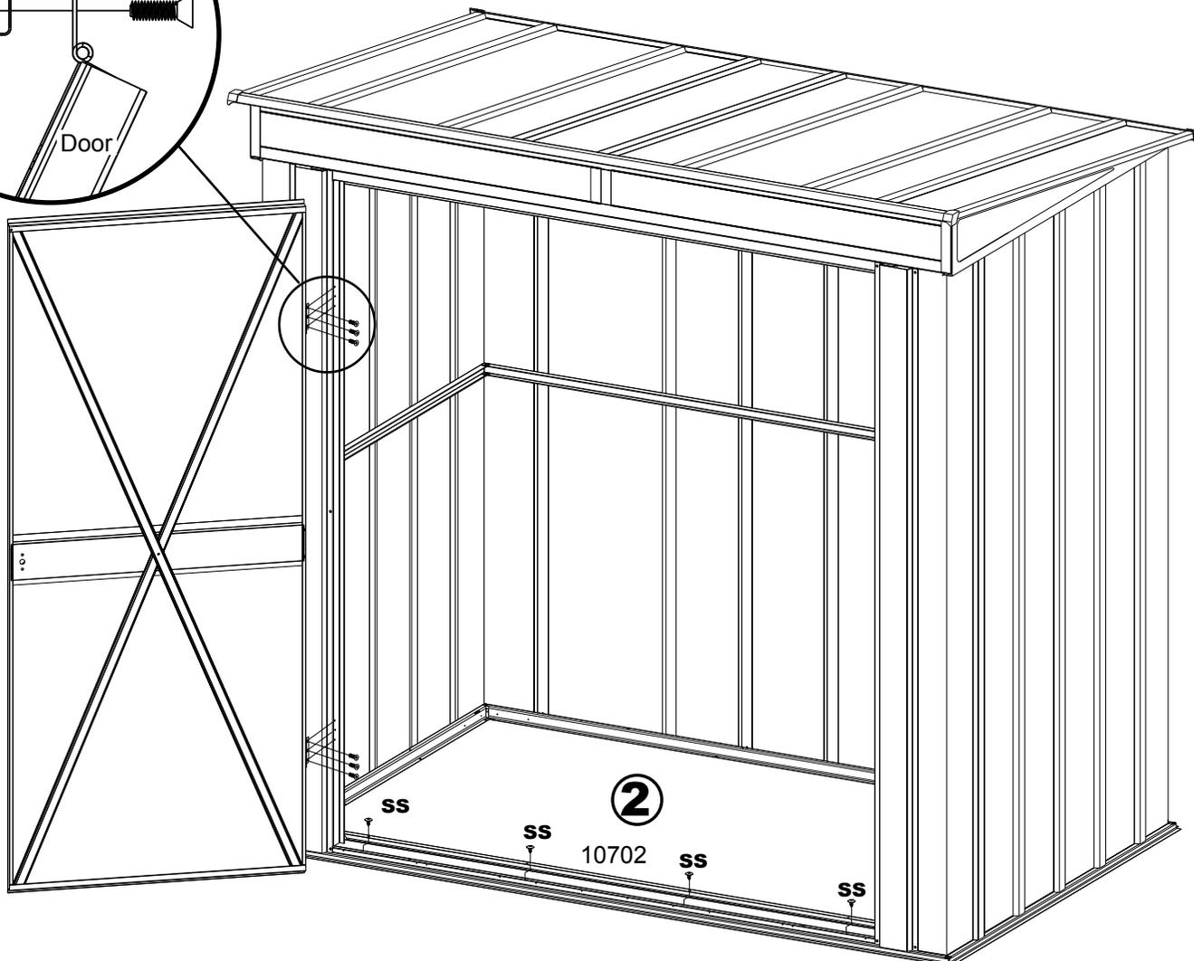
**2** Fasten Ramp to Floor Frame using four (4) Sand Screws.
