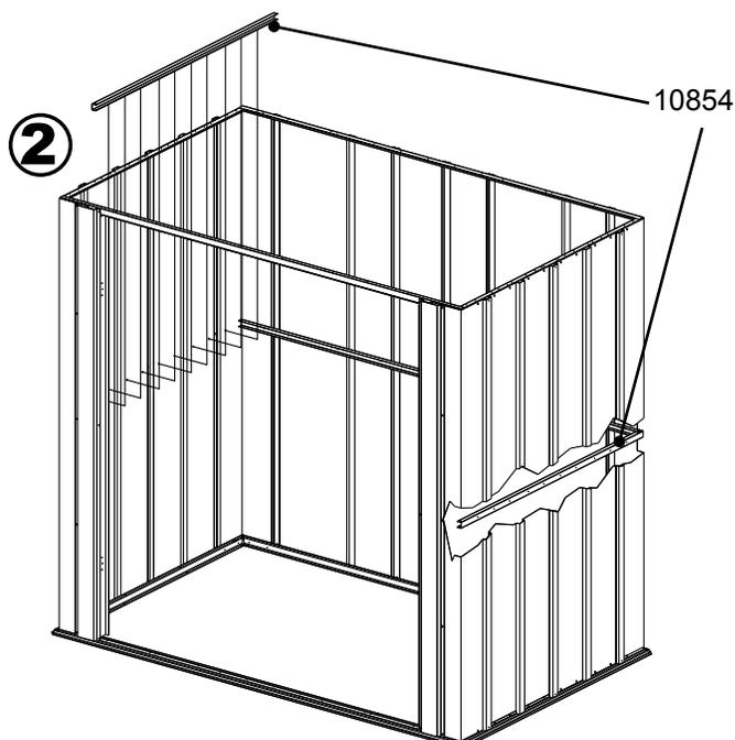
**2** Install **Side Wall Channel** by placing **Sand Screws** through all remaining holes in **Side Wall Panels**.
