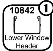
**1** Attach **Lower Window Header** to the **Front Header** using ten (10) **Sand Screws** as shown. Leave holes #3, #5, #10, and #12 open at this time.
