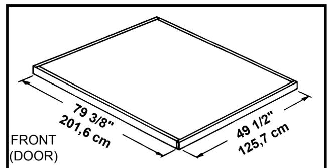
Note: Finished Slab dimensions, with lumber removed.
