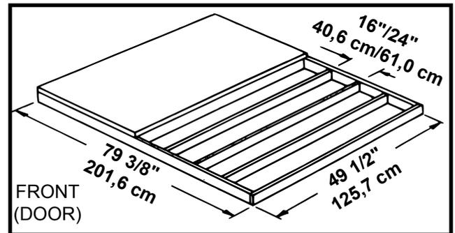
Note: Platform/Slab will extend 9/16" (1,4 cm) beyond floor frame on all four sides. Seal this 9/16" (1,4 cm) of wood with a roofing cement (not included), or bevel this 9/16" (1,4 cm) of concrete when pouring, for good water drainage.
