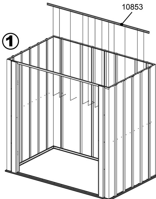
**1** Install **Rear Wall Channel** by placing **Sand Screws** through all remaining holes in **Rear Wall Panels**.
