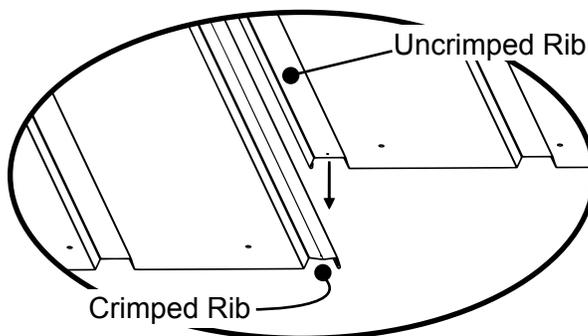
Whenever a crimped rib and an uncrimped rib meet, place the crimped rib **UNDER** the uncrimped rib.
