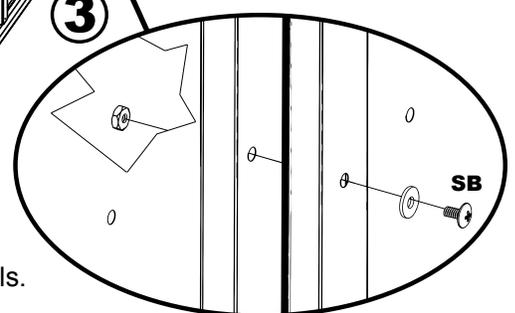
Attach Wall Panels with screws through all holes in top and bottom of Panels.
