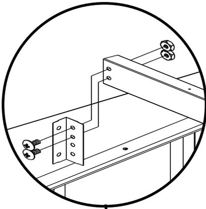
Attach Roof Beam to Gable Brace through top two (2) holes.
