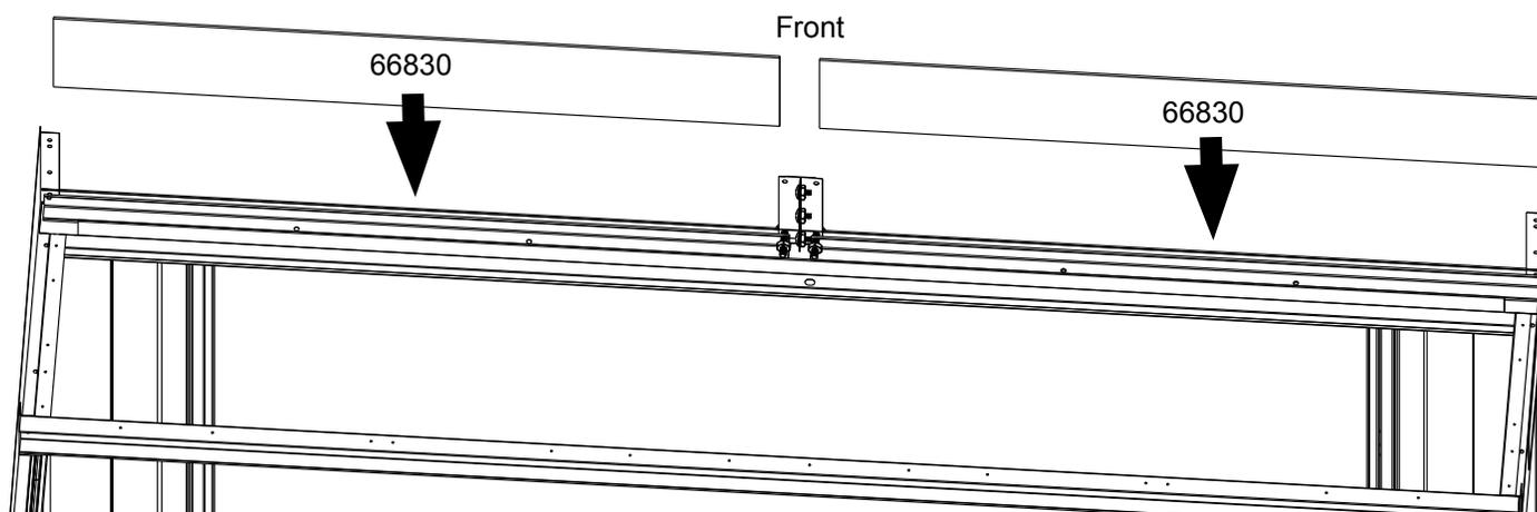
**6** Secure **Window Support Angle Lower** to **Window Header Lower** using four (4) **Sand Screws** as shown. See diagram below.
