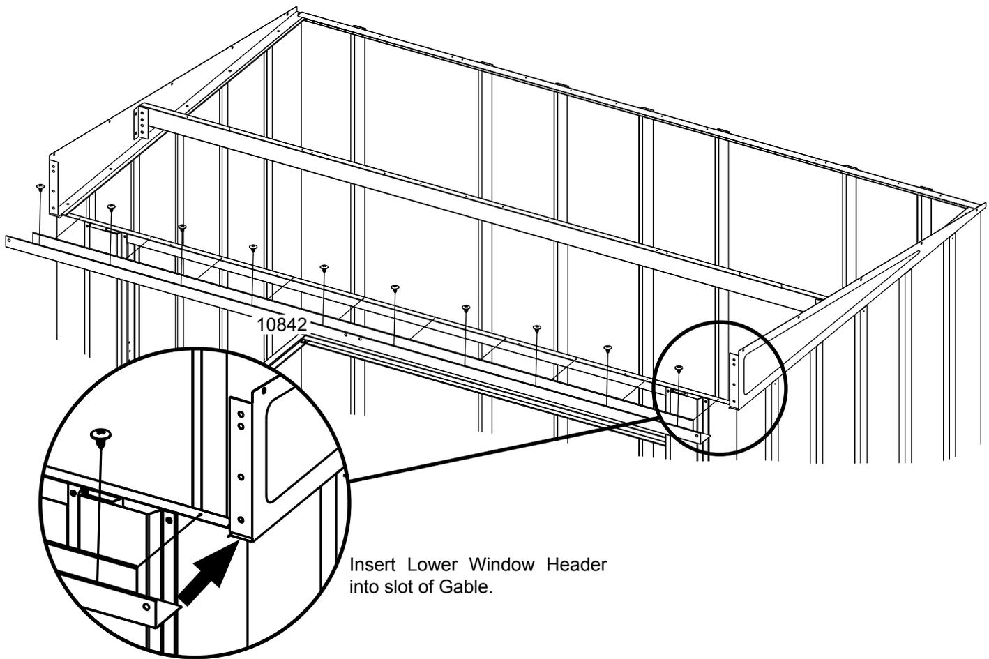
Insert Lower Window Header into slot of Gable.
