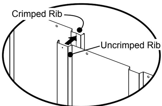
Whenever a crimped rib and an uncrimped rib meet, the crimped rib should be placed **UNDER** the uncrimped rib if possible.
