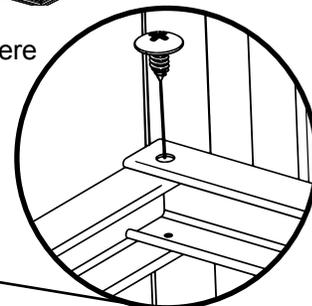
**3** Insert a **Sand Screw** in both rear corners where **Side** and **Rear Wall Channels** meet.
