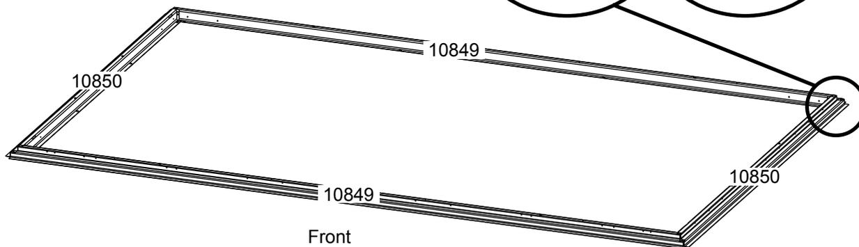
When diagonal measurements are equal, the Frame is square.
