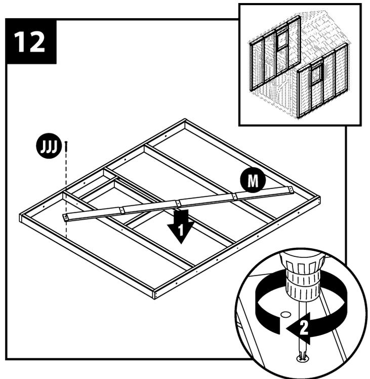
Measure from one upper corner to the opposite bottom corner. The measurement should be close to 117 5/8". The exact measurement is not as important as having the same distance when you measure the opposite corners. Tack the temporary brace in place once the diagonal measurements are equal. The brace should remain in place until it interferes with adding more siding. The squareness of the frame should also be checked with a carpenters square.
