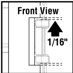
**Note:** Tack the side trim in place, **DO NOT** permanently nail the parts until the top trim piece has been fitted using 2" 6-Penny finish nails (GGG).
