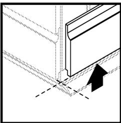
Line up the ends of the back wall's first piece of siding with the siding on the side walls. It is much more important that the first piece be level.
