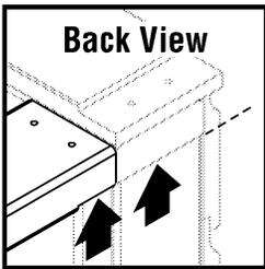
Using a carpenter's square, insure that the back wall's upper corners are both 90°.
