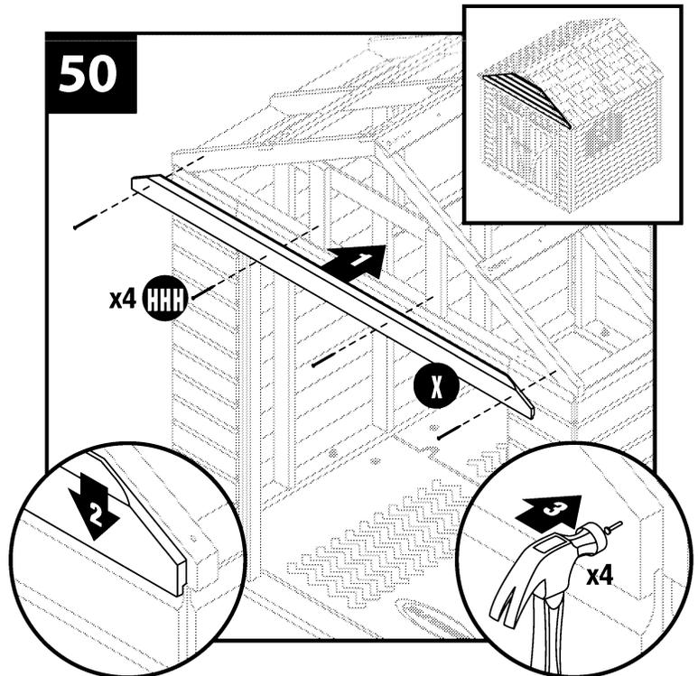
Add the narrowest 46 1/2" gable siding (AA) on top using (4) 2 1/4" 6-Penny nails (HHH).
