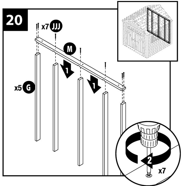
Finish the back wall framing by adding the second 84" back wall top and bottom plate (M) to the opposite ends of the studs using (7) #10 x 3" deck screws (JJJ).
