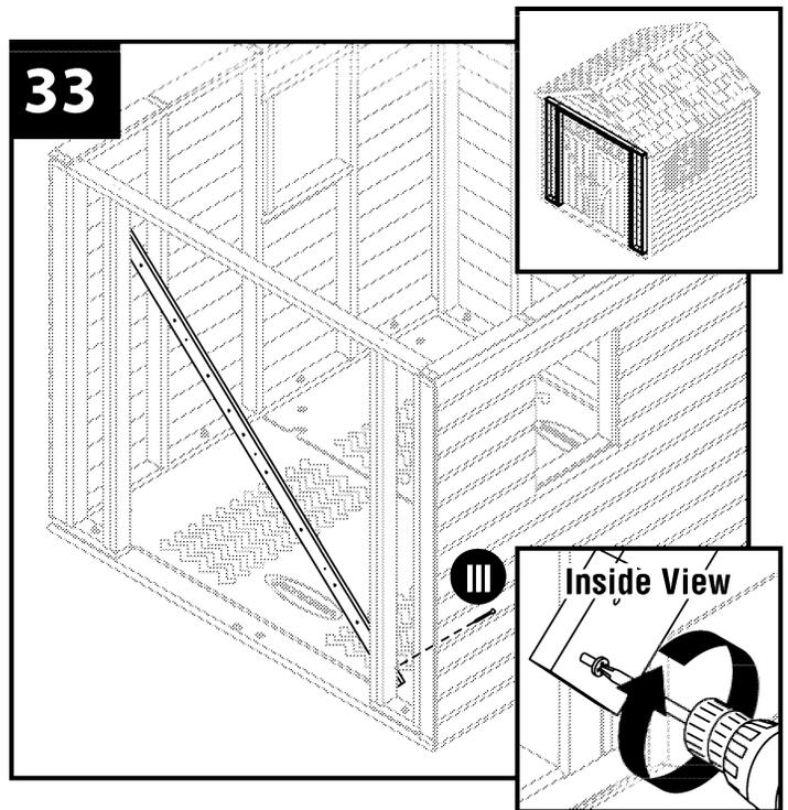
Once you are certain that the door opening is true, the front wall can be fastened to the side wall's end studs using (4) #10 x 3" deck screws per side.
