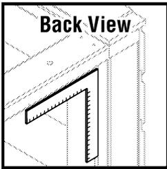
If the back wall is not lining up with the side wall, or the upper corners are not at 90°, a rafter (O) should be used as a brace to temporarily force the back wall frame to remain square until it is attached to the side walls.
