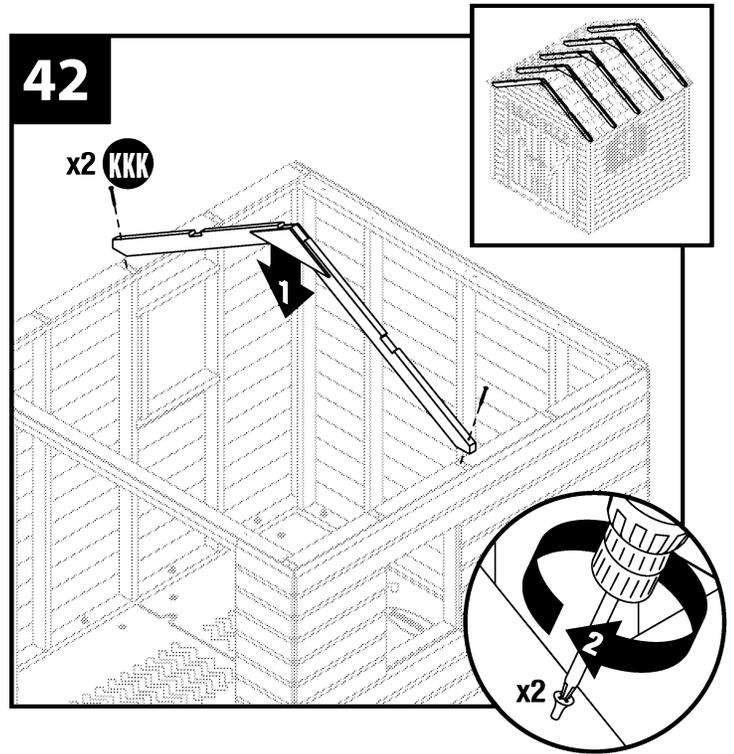
Repeat the mounting process for the remaining four rafter assemblies. Remember, the front and back rafters only have one gusset and that the gusset should face the interior of the shed (The vent will eventually take up the position where the second gusset would be).
