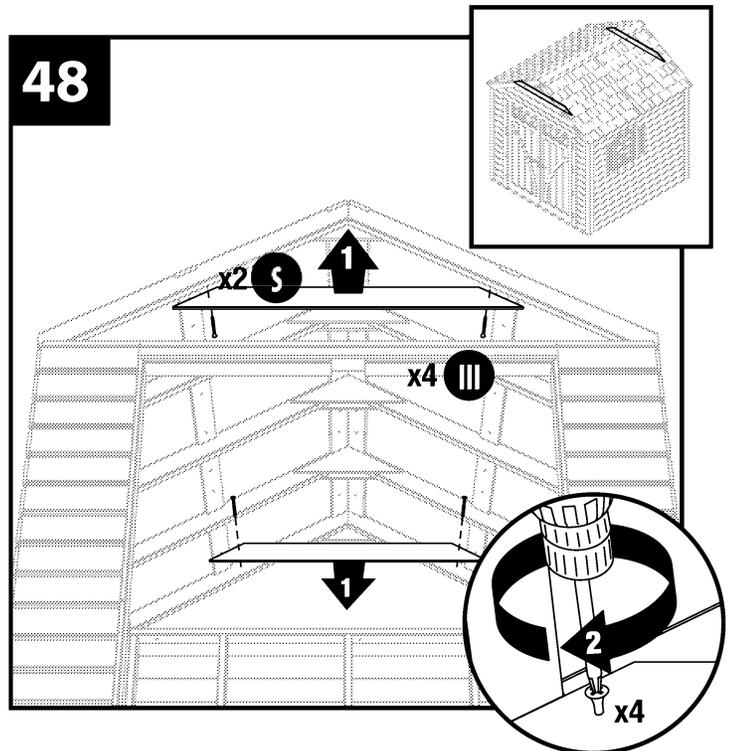
Two pieces of 2" x 4" bracing are added to the gable ends to provide a fastening surface for the gable end siding. Fasten (2) vertical gable braces (R) in front of each gable brace (S) with (4) #10 x 2" deck screws (III).
