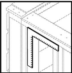
**Note:** It may be necessary to loosen the front wall's J-bolts (Step 31) while squaring-up the door opening. It is recommended that the door opening remain braced until the front siding has been applied.
