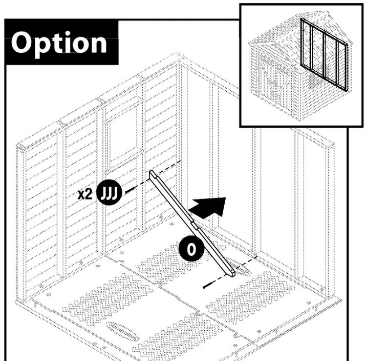
Secure the side wall to the back wall frame using (4) #10 x 3" deck screws (JJJ).
