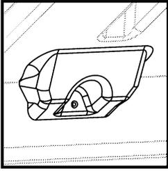
Install (4) #8 x 3/4" washer head screws (DDD) through the molded locations into the fascia.
