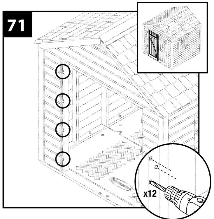
Fasten the doors to the door frame with (3) #8 x 1 1/4" wood screws (FFF) at each hinge location.
