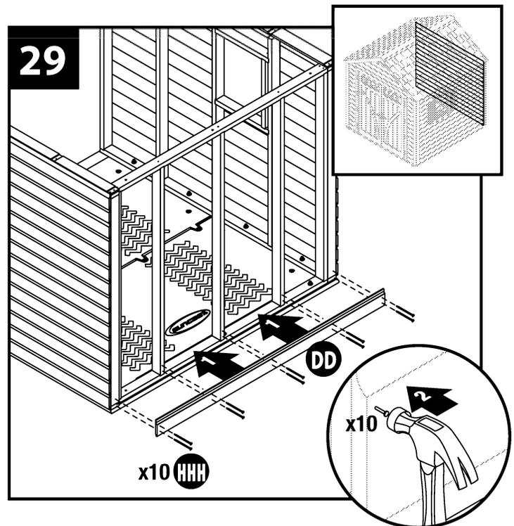
Secure each following piece of 91" siding (DD) with (10) 2 1/4" 6-Penny nails (HHH) being sure to nail through the thicker part of the siding and into the 72" studs behind them. Try to keep the siding level to the floor and even with the siding pieces on the side walls at each end.
