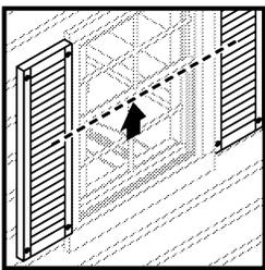
**Caution:** Do not screw into the thin part of the siding. Move the shutter up or down until the holes line up with a full piece of siding.
