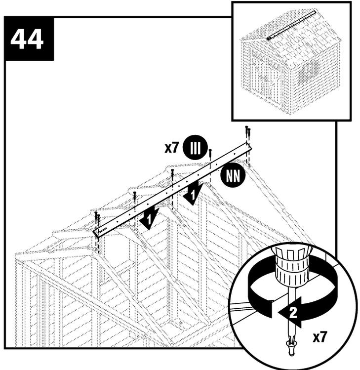
Match a roof lathe (NN) on the other side of the peak. Fasten through the holes provided into the rafters with (7) #10 x 2" deck screws (III). Two screws are used at each end of the lathes and a single screw each into the middle three rafters.
