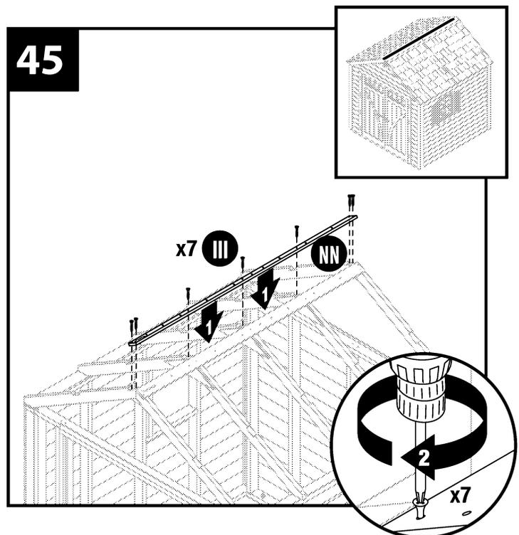
Add third roof lathe (NN) midway down rafters. Fasten through the holes provided into the rafters with (7) #10 x 2" deck screws (III). Two screws are used at each end of the lathes and a single screw each into the middle three rafters.
