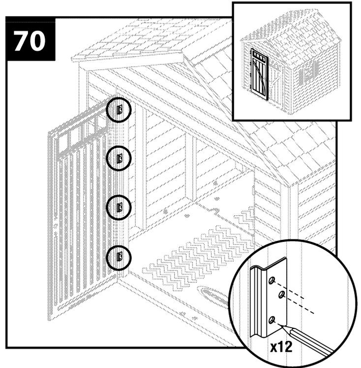
Pre-drill each marked hole location with a 1/8" drill bit (total of 12 holes). Drill approximately 1" deep.
