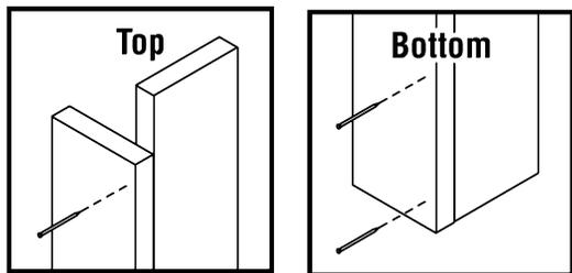
Attach to the shed so that the outside corner of the gable trim matches the outside corner of the corner trim assembly. Nail into place using (10) 2" 6-Penny finish nails (GGG). Repeat the process for the back wall corner trim pieces.
