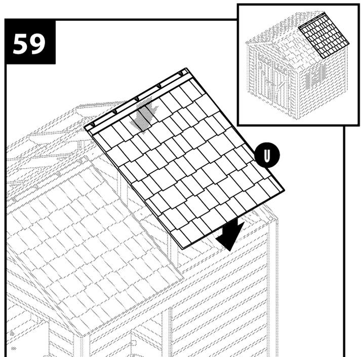
Once the (2) right roof panels are in place, they should be fastened first into the roof lathe at the ridge. Screw (10) #8 x 3/4" washer head screws (DDD) through the outside of the roof panels and into the lathe.
