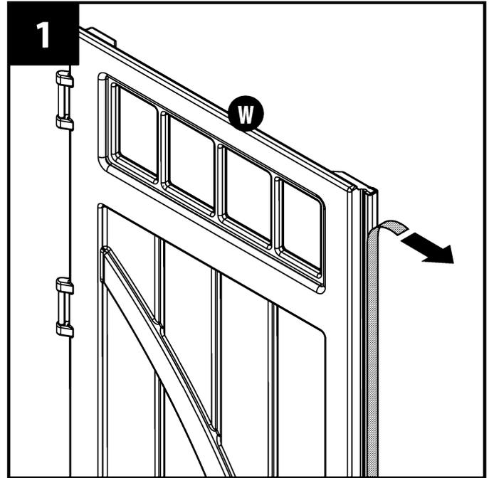
Peel film from both sides of door window (HH). Stand left door (W) vertically. With at least two people (one person on each side of door), layer into door channel first the door window gasket (JJ), then the door window (HH). Through the back of the door, secure layers with (11) #8 x 1/2" washer head screws (CCC) (start with four corner screws and then finish with remaining screws). **DO NOT** over tighten screws. Repeat on right door (V).
