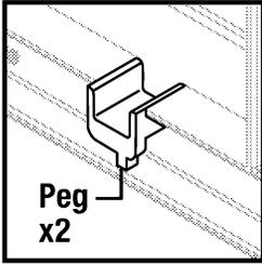
Pull screen (P) onto 2 pins in corners and stretch screen up over top pin.
