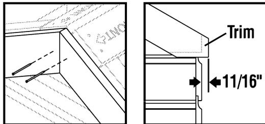
**Note:** The upper extent of the gable trim is unsupported, and should be backed-up with a small piece of extra siding to prevent damage to the plastic vent component. One trim nail to each side of the center joint will hold the formed peak.
