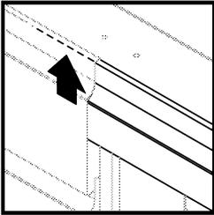
Make sure that the siding-over-door (CC) does not fall below the bottom surface of the door header. You should be able to see the bottom of the door header below the bottom of the siding-over-door (CC).
