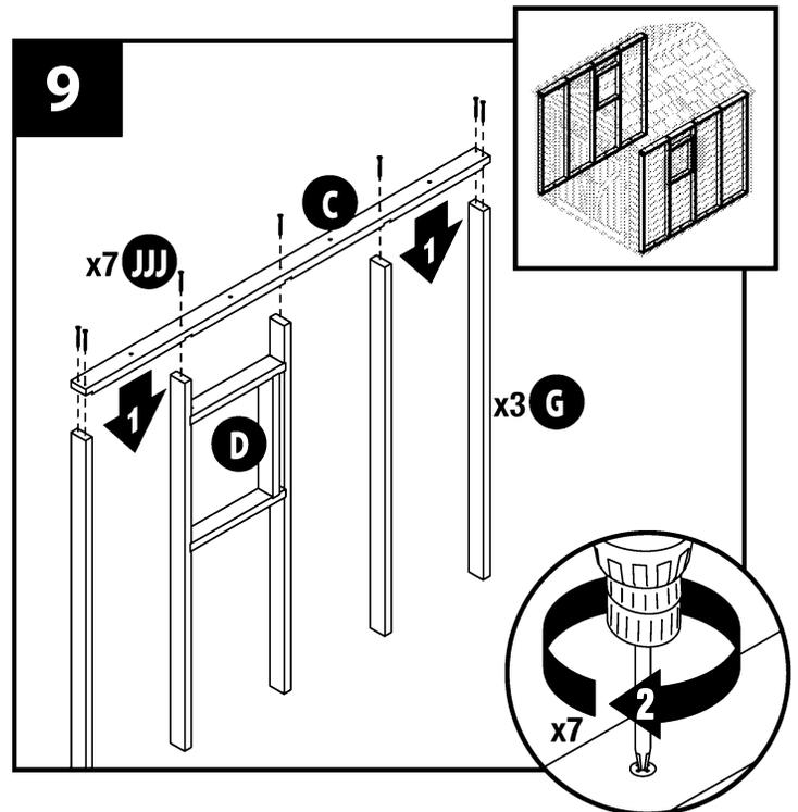
To finish the basic stud wall, attach the top/bottom plate (C) using (7) #10 x 3" screws (JJJ).
