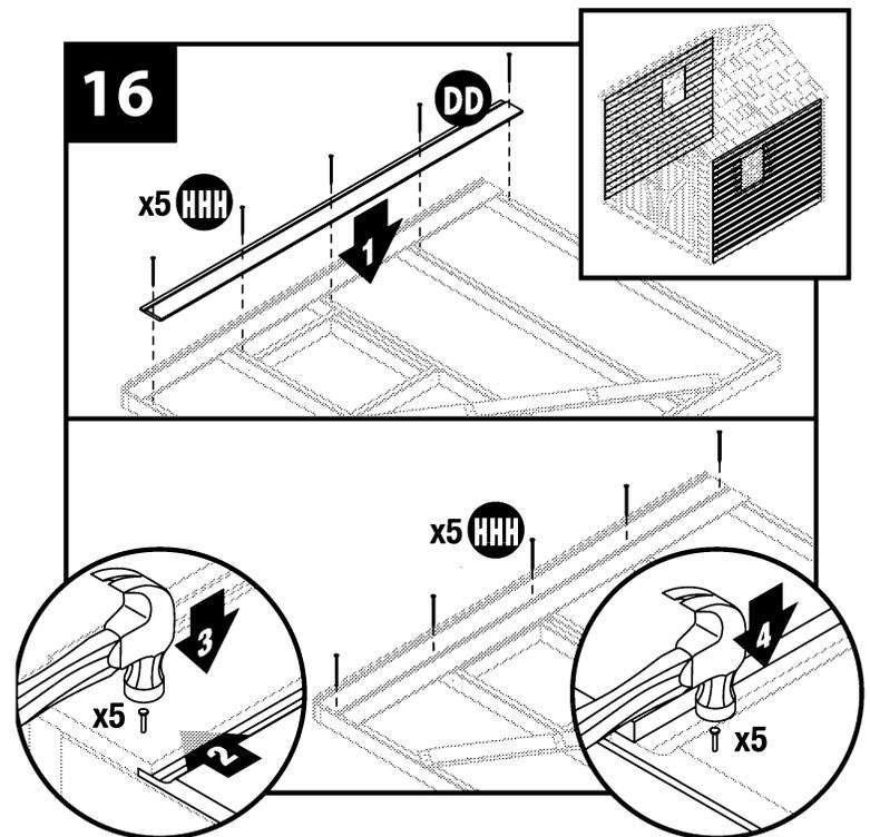
Siding around the windows is accomplished in a similar fashion. The 23 1/4" window siding (EE) will fit to one side and the 48 1/4" window siding (FF) will fit to the other side. Add these siding strips in the same manner as the first full length strip, tapping them up underneath the strip above and adding a second row of nails (HHH) to the top edge of the second strip and nailing only the top edges first.
