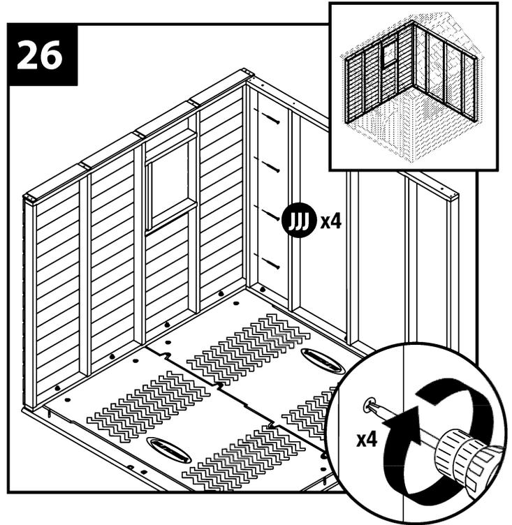
Carefully place the 2nd side wall onto the floor making sure that the protruding J-hooks (YY) are coming up through the holes in the bottom plate. Using (4) J-hook washers (ZZ) and (4) J-hook nuts (AAA), secure the side wall to the floor.
