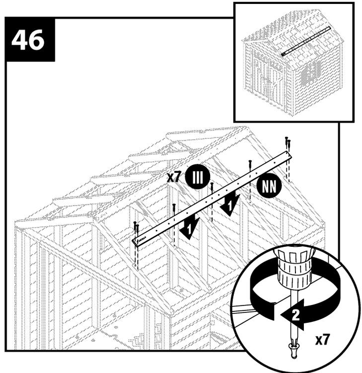
Add fourth roof lathe (NN) midway down rafters. Fasten through the holes provided into the rafters with (7) #10 x 2" deck screws (III). Two screws are used at each end of the lathes and a single screw each into the middle three rafters.
