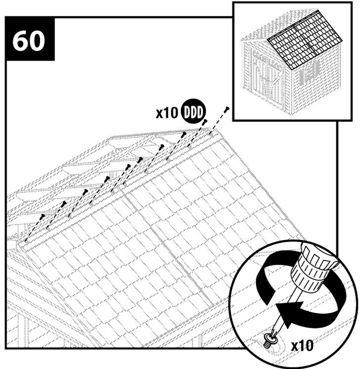
There are four screw locations molded into each roof panel for attaching to the fascia.
