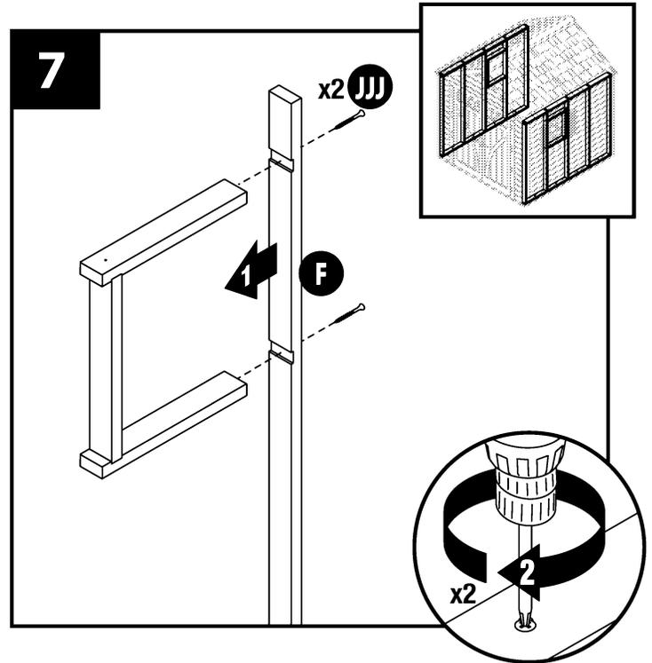
Attach a second 72" stud with window detail (F) to the opposite side of the window opening using (2) #10 x 3" deck screws (JJJ).
