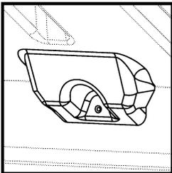
Install (8) #8 x 3/4" washer head screws (DDD) through the molded locations into the fascia.
