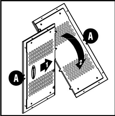
Fasten the two floor panels (A) together to complete floor assembly using (4) 5/8" pan head screws (BBB).
