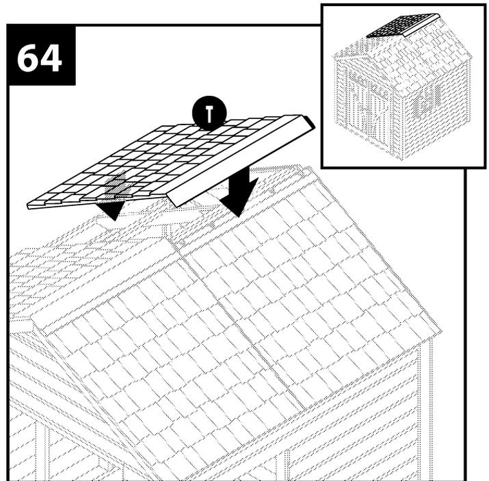
The left roof panels can then be fastened to the ridge roof lathe.
