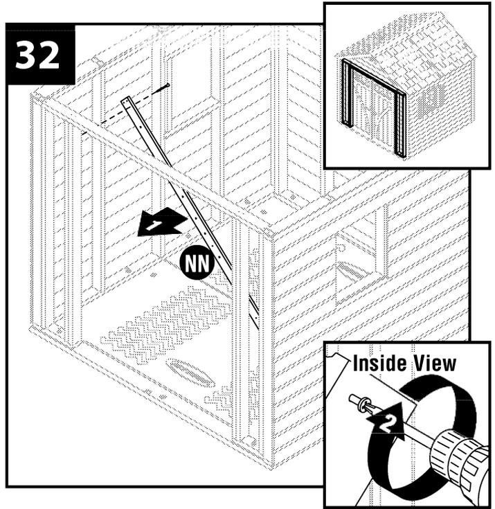
The other end will be tacked into place once the upper corners of the door opening have been checked with a carpenter's square.
