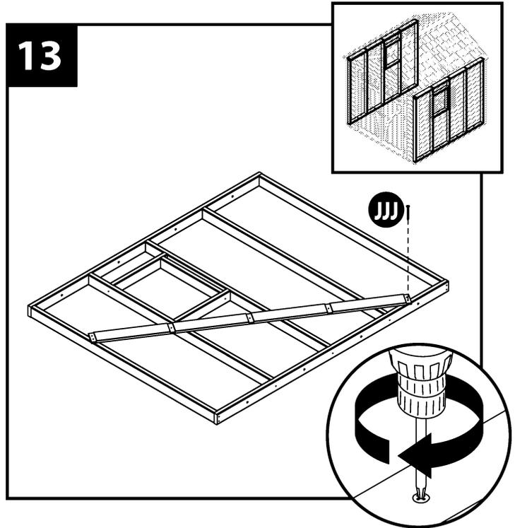
The soffit in this view would put the window toward the front if used on the RIGHT and toward the back of the shed if used for the LEFT wall. The 91" soffit and rafter support (B) is screwed down with the (7) #10 x 2" deck screws (III).
