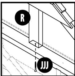
For the front braces, the door header should be temporarily removed.
