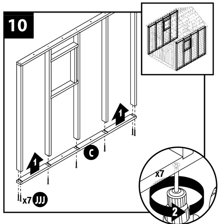
Decide on one of two positions for the window on a particular side wall. Until the soffit and rafter support (B) is added, the framed wall can be flipped over to bias the window toward the front or the back of the shed.
