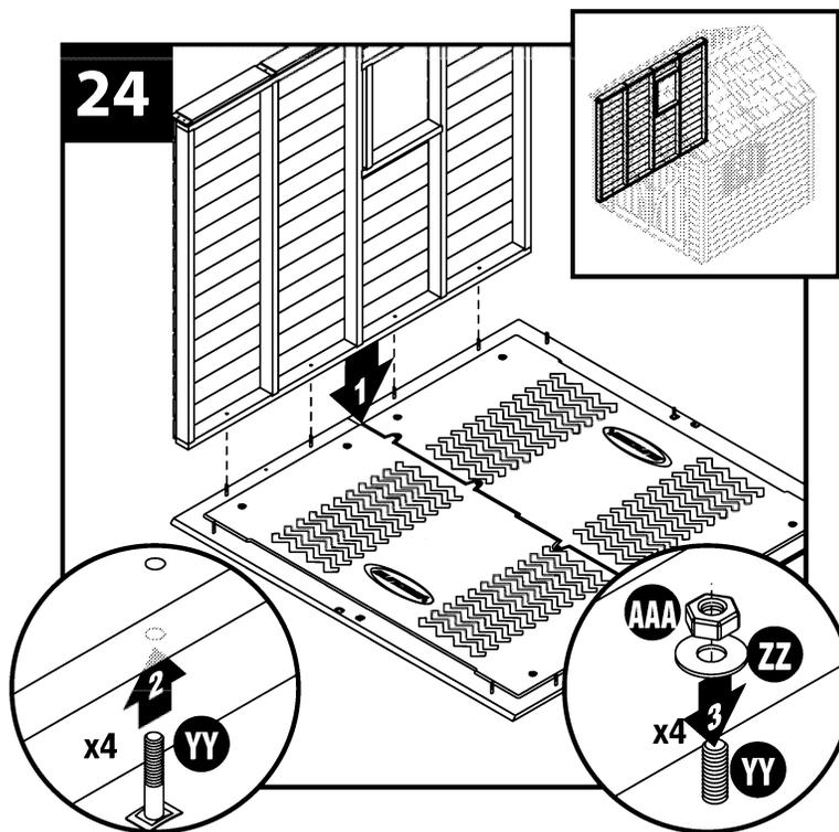
Carefully place the back stud wall onto the floor making sure that the protruding J-hooks (YY) are coming up through the holes in the bottom plate. Using (3) J-hook washers (ZZ) and (3) J-hook nuts (AAA), secure the back wall to the floor.
