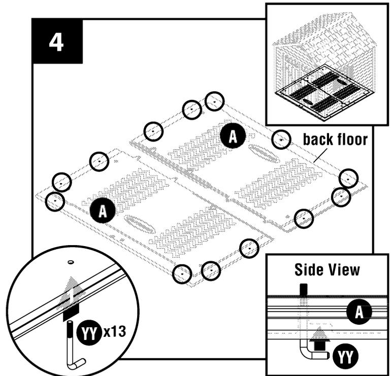
The floor panels (A) must be brought together as shown below.
