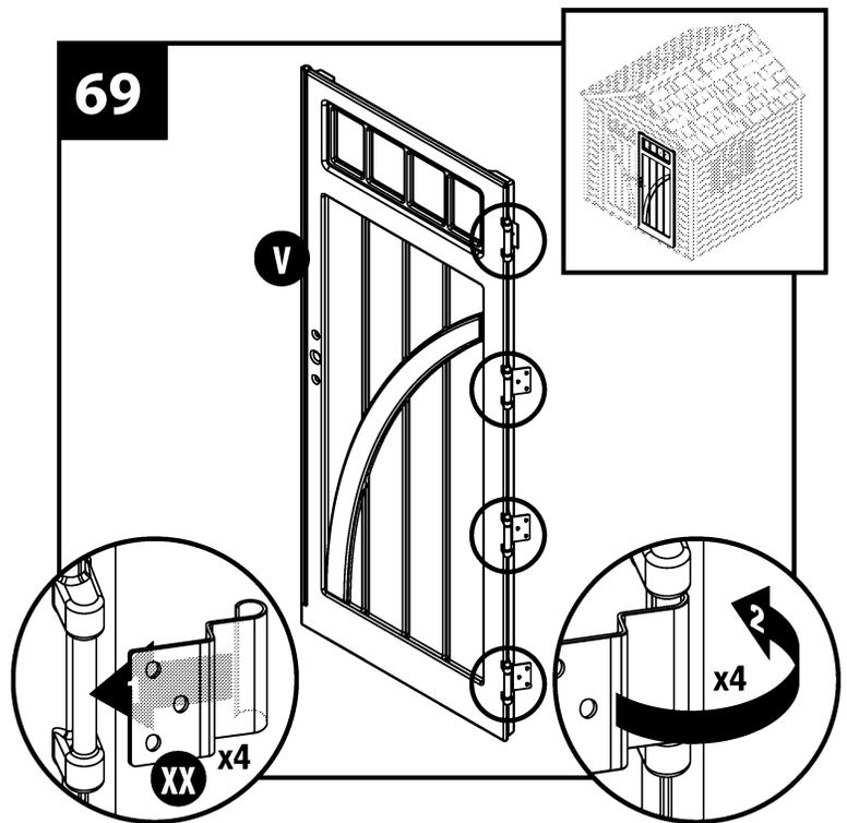
Hold the left door (W) up to the left door post and match the top of the upper hinge to the mark made in Step 68. Mark the location of the holes for each hinge (12 holes).
