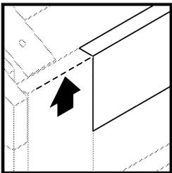
Once in place, each fascia board is nailed in place with (9) 2" 6-Penny finish nails (GGG) going into the rafter ends and the edge of the soffit. Repeat for opposite side fascia.
