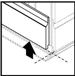
The inside edges should be 3/4" from the door opening to allow room for the door hinges.
