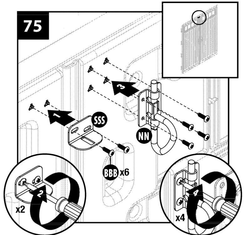
At the bottom interior side of right door, attach remaining clip (SSS) with (2) 5/8" pan head screws (BBB) through provided holes.
