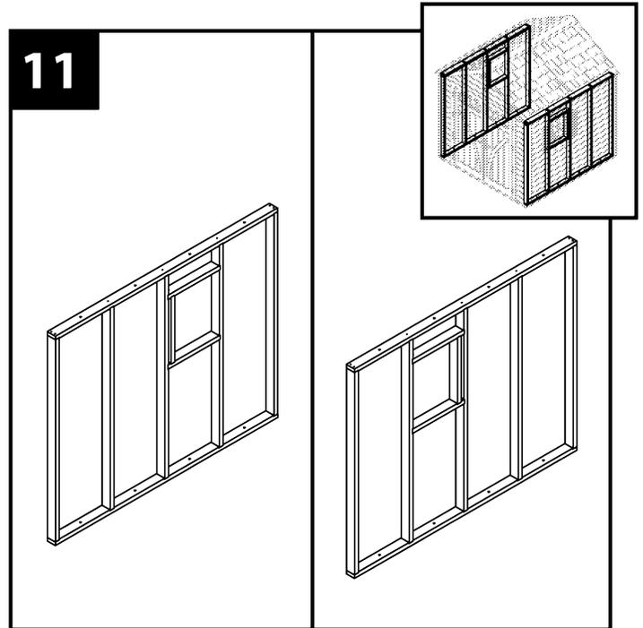
Lay frame on a flat surface. Square up the framed side wall using a 84" top/bottom plate (M) as a temporary brace. Tack one end of the board to an end stud, using a #10 x 3" deck screw (JJJ). The other end of the board will be tacked into the side wall's bottom plate once the wall has been squared up.
