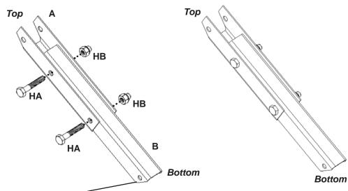
Angled end of Truss Bracket B (B) faces down.
