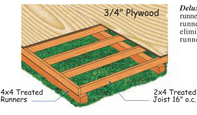
**Deluxe Floor (optional accessory):** 4x4 treated runners can be installed directly on the grass. The runners elevate the floor providing air flow eliminating moisture. 10' wide floor has three runners. Floor covering is 3/4" plywood.
