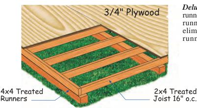
**Deluxe Floor (optional accessory):** 4x4 treated runners can be installed directly on the grass. The runners elevate the floor providing air flow eliminating moisture. 12' wide floor has four runners. Floor covering is 3/4" plywood.
