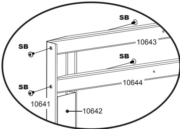
**5** Next, insert the **Upper/Lower Chord Truss Assembly** into the **Truss Post Assembly** as shown. Secure with **Small Bolts and Nuts**. Do not tighten at this time. Repeat for other side.
