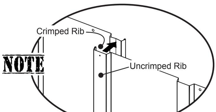
Whenever a crimped rib and an uncrimped rib meet, the crimped rib should be placed UNDER the uncrimped rib if possible. See next page.
