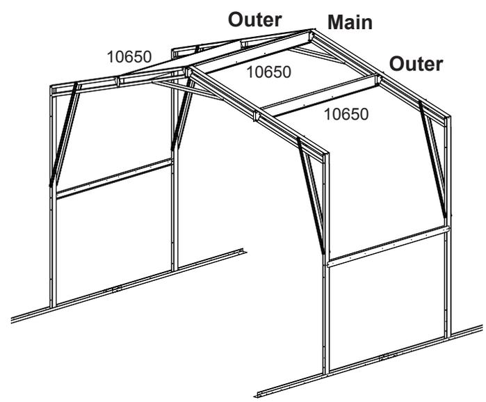
**3** Remove Bolts holding Truss peaks together (from Step 1-6). Next, place two **Middle Roof Beams** back-to-back and secure with two **Small Bolts and Nuts** as shown above. This is the **Main Roof Beam**.
