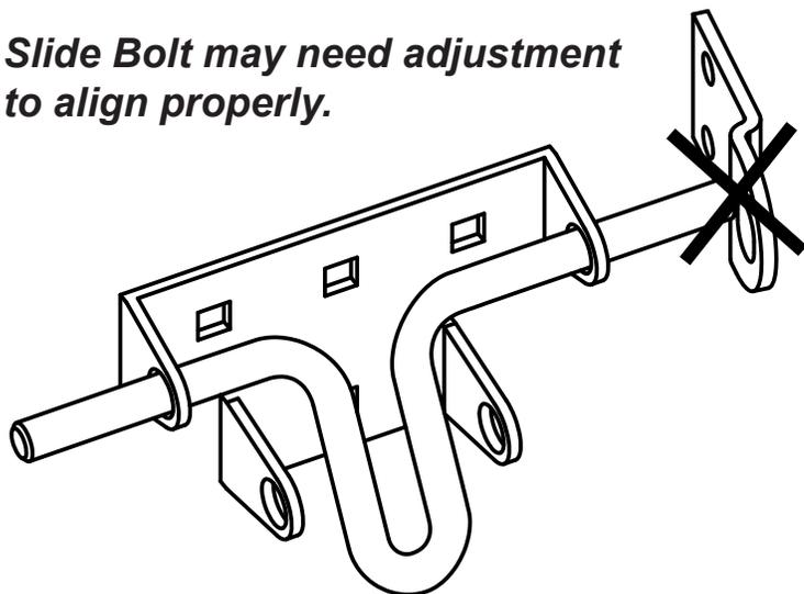
If Slide Bolt does not align properly, you may need to insert plastic washers between the door and the Slide Bolt to ensure proper fit. Adjust number of plastic washers until desired fit is reached.
