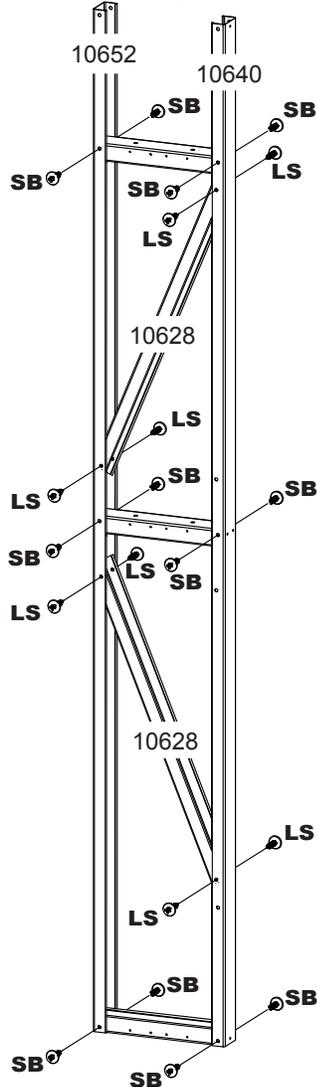
**1** Lay out the parts and position them as shown. Double check that holes align as shown. If holes do not align, the **Wall Post (Hinge)** is most likely upside-down.
