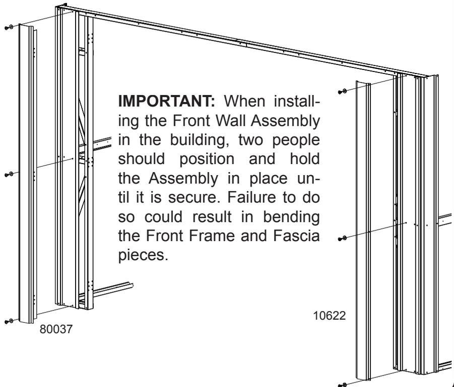
**1** Just as in the rear, carefully position the **Front Wall Assembly** as shown and secure with a **Large Screw** on both sides. Install **Front and Rear Side Wall Channels** using **Large Screws**.
