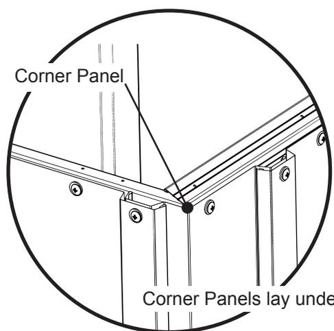
Corner Panels lay under Front and Side Panels.
