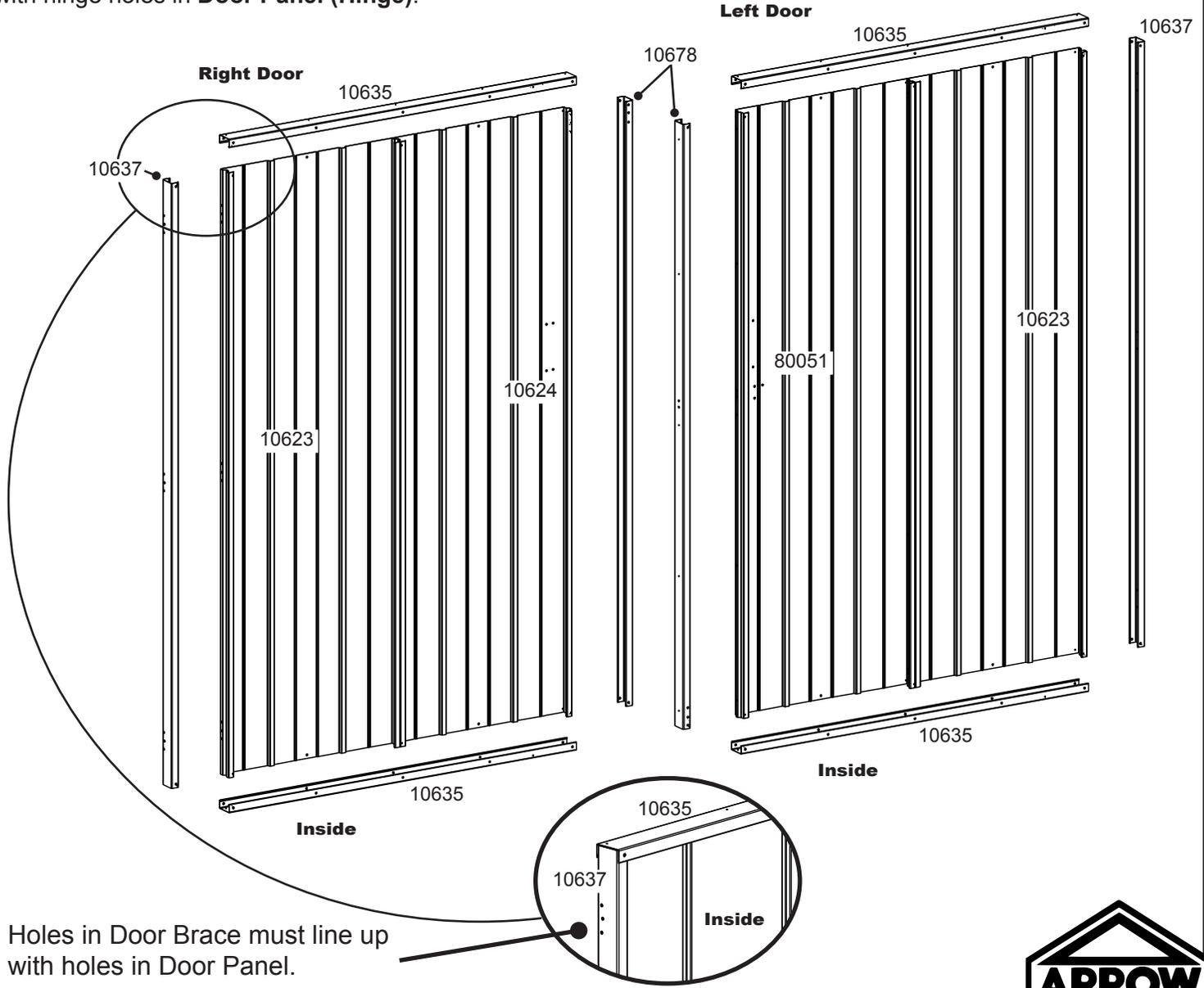
Holes in Door Brace must line up with holes in Door Panel.
