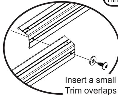
Insert a small screw where Roof Trim overlaps after installing.
