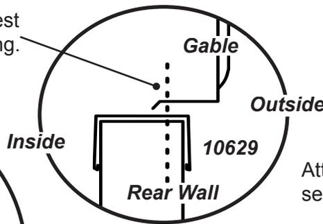
Attach Brace with bolt thru second hole from bottom only.
