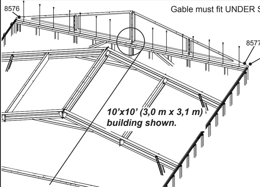
Gable must fit UNDER Side Wall Angle at corner.
