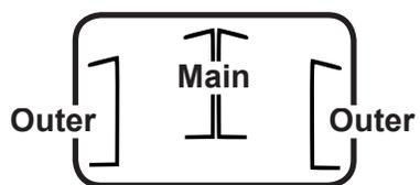
*Side of beams with small holes must face up.*
