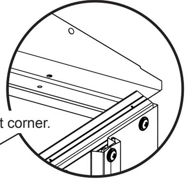
**2** Working with one **Gable** at a time, attach the **Gables** to the top **Rear Frame** with **Small Screws**. The **Gable** should be attached using the row of holes closest to the outside of the building. Do not insert screws into the two holes closest to where the **Gables** join. These will be used to attach the **Track Support** later.
