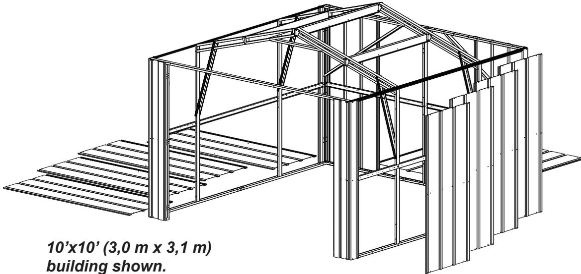
**1** Working one side at a time, lift the **Panels** into place and secure top and bottom of **Panels** with **Small Screws**. Be sure to overlap ribs as shown on the previous page.
