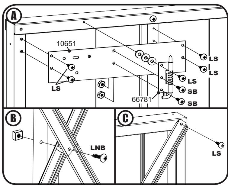
**4** **A:** Position parts as shown and secure to upper inside corner of left **Door** with **Large Screws**. **Spring Latch** attaches to **Latch Plate** using **Small Bolts and Nuts**. Place three **Plastic Washers** behind top hole of **Spring Latch** as shown; this will help alignment.
