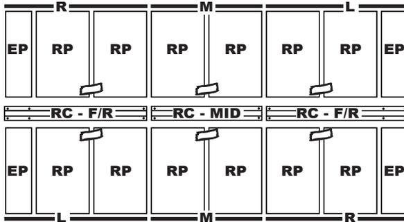
**NOTE:** The symbol
