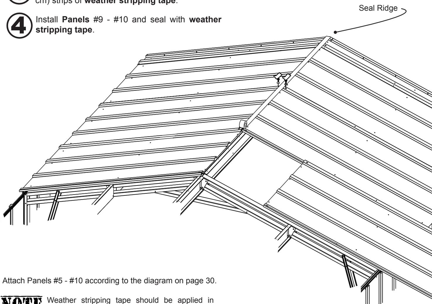
Attach Panels #5 - #10 according to the diagram on page 30.
