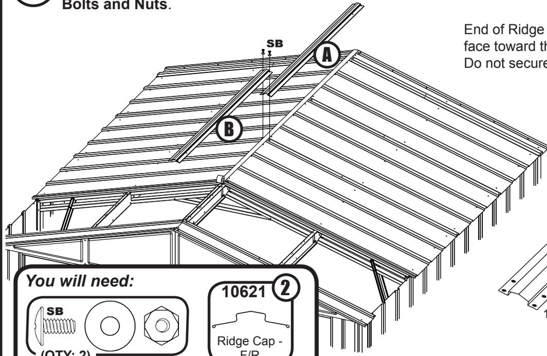
End of Ridge Cap with four holes must face toward the outside of the building. Do not secure at this time.
