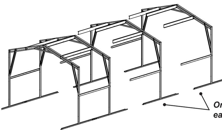
**5** All Truss Sections are assembled in the same manner as the Truss Section just erected. Install one additional Side Frame per side for each additional Module. Overlap Side Frames by 8 1/4" (21,0 cm). Refer to page 13 to see how many Trusses should be included in your building.
