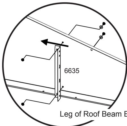
Leg of Roof Beam Bracket must face center of Gable as shown.
