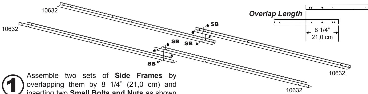
**1** Assemble two sets of **Side Frames** by overlapping them by 8 1/4" (21,0 cm) and inserting two **Small Bolts and Nuts** as shown above. These will form the left and right **Floor Frames**.
