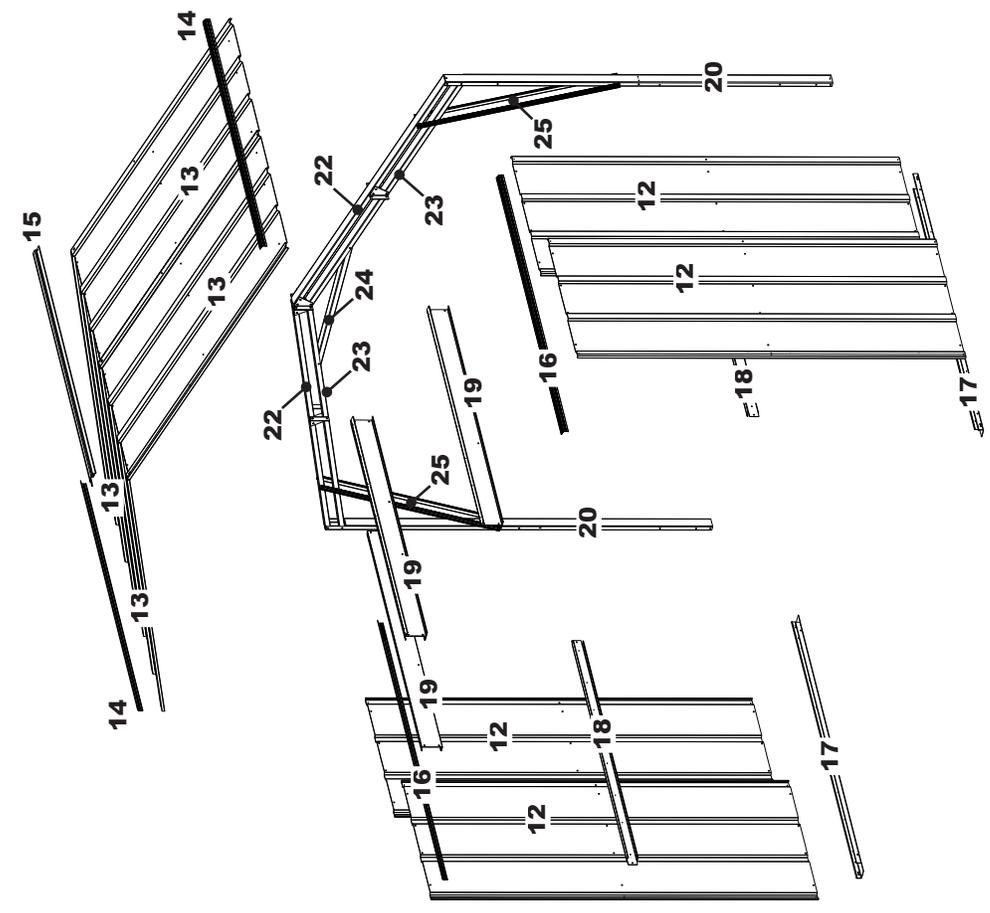
**NOTE** Part No. 21 (Truss Post Insert) fits inside Part No. 20 (Truss Post) and is not shown above.
