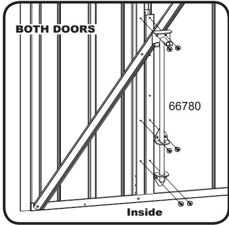
**5** Secure all **Diagonal Braces** to the **Vertical Door Braces** with **Large Screws** as shown. Next, position the **Cane Bolt Bracket** back-to-back against the **Vertical Door Brace** closest to the center of one **Door** as shown. Slide the **Cane Bolt Bracket** to the bottom of the **Door** and secure with three **Large Screws**. Repeat for other **Door**.
