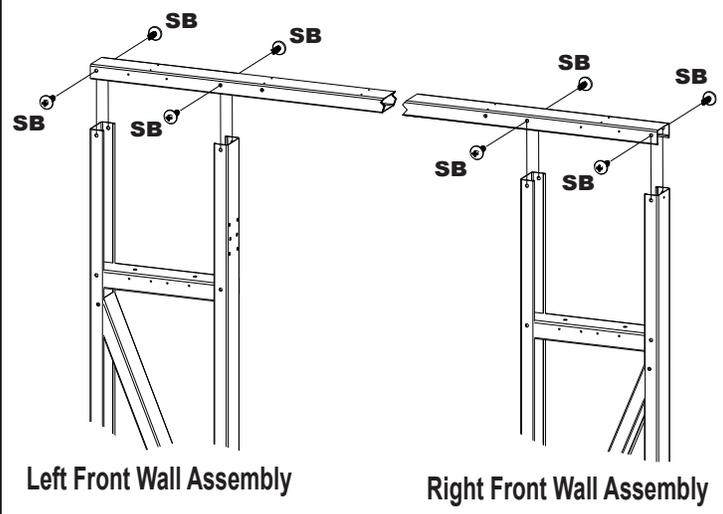
**5** Slide the **Door Header Assembly** down onto the **Front Wall Assemblies** as shown and secure with **Small Bolts and Nuts**. Once these pieces are joined, take care when moving them as the **Door Header** may bend.
