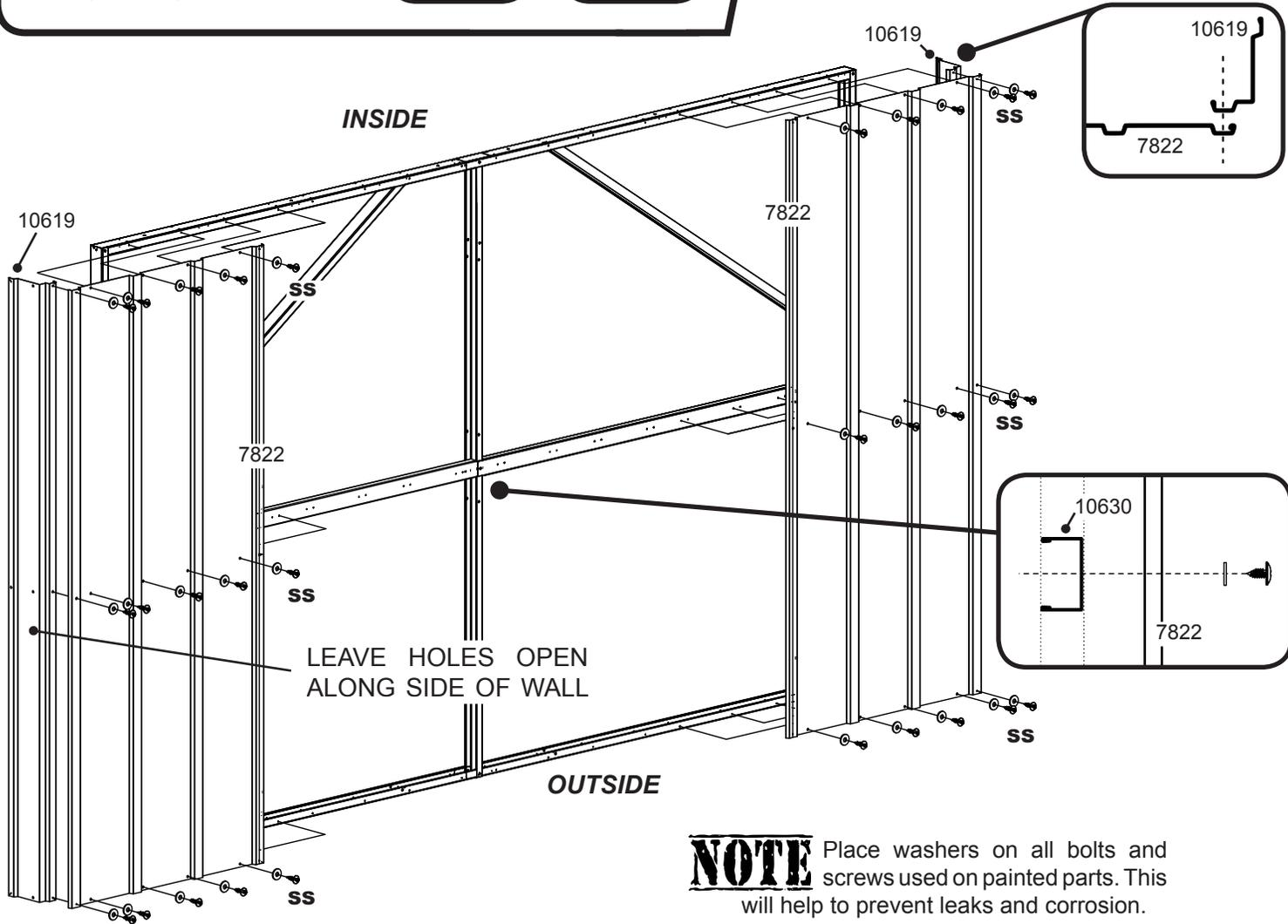
**NOTE** Place washers on all bolts and screws used on painted parts. This will help to prevent leaks and corrosion.
