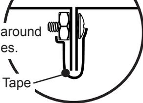
Tape BOTH Gable joints before installing Roof Beams.
