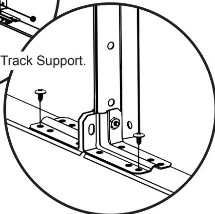
**4** Position **Track Supports** as shown. Secure **Track Supports** to **Gable** using one **Small Bolt and Nut**. Secure to **Rear Frame** using two **Small Screws**.
