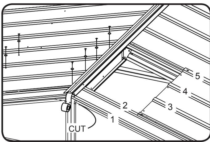
**NOTE** DO NOT fully tighten Ridge Cap bolts until you have both Ridge Cap bolts in place. This will ease assembly. Bolts must be fully tightened before moving on to the next page.
