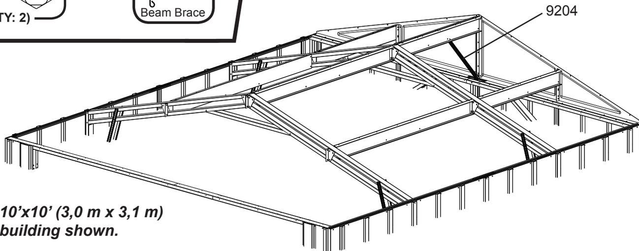
**8** Attach the **Roof Beam Brace** to the **Track Support** with one **Small Bolt and Nut** as shown.
