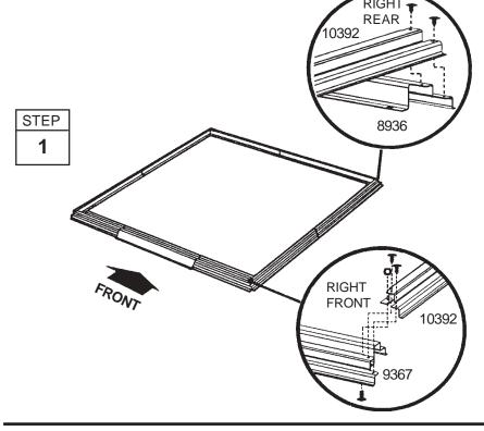
**2** Measure the floor frame diagonally. When the diagonal measurements are equal, the floor frame is square.
