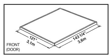
Note: Finished Slab dimensions, with lumber removed.
