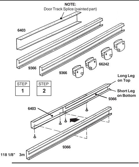
**3** Position door slides onto the legs, from the end of door track assembly, as shown in the end view. NOTE: Flat side on top, pins and holes <u>must</u> be oriented as shown.
