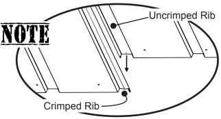
Whenever a crimped rib and an uncrimped rib meet, place the crimped rib UNDER the uncrimped rib.
