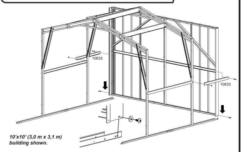
Carefully position the **Rear Wall Assembly** in place at the rear of the building and secure to Side Frame with one **Large Screw** per side as shown.
