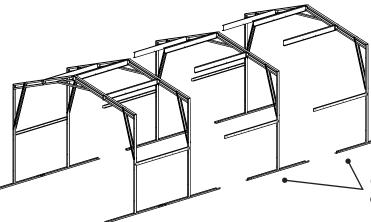
All **Truss Sections** are assembled in the same manner as the **Truss Section** just erected. Install one additional **Side Frame** per side for each additional Module. Overlap **Side Frames** by 8 1/4" (21,0 cm). Refer to page 13 to see how many **Trusses** should be included in your building.
