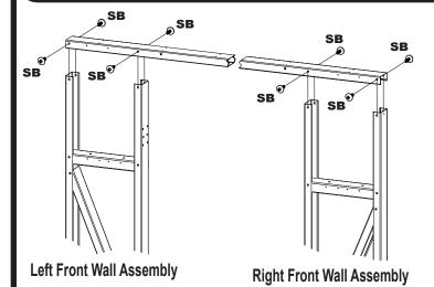
Slide the **Door Header Assembly** down onto the **Front Wall Assemblies** as shown and secure with **Small Bolts and Nuts**. Once these pieces are joined, take care when moving them as the **Door Header** may bend.
