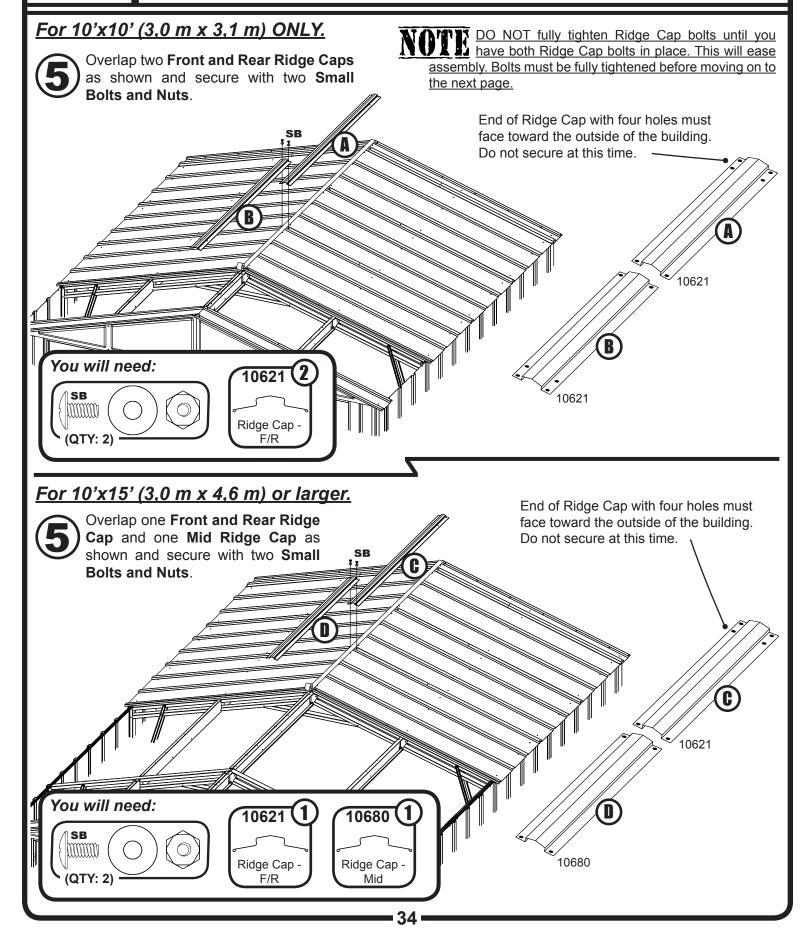
DO NOT fully tighten Ridge Cap bolts
