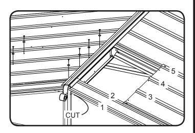
DO NOT fully tighten Ridge Cap bolts until you have both Ridge Cap bolts in place. This will ease assembly. Bolts must be fully tightened before moving on to the next page.
