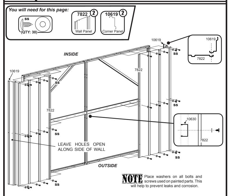
Using Small Screws, attach a Wall Panel and Corner Panel to each corner of the Rear Wall as shown. The Corner Panel should only be secured to the Wall Panel where the panels overlap. Do not secure the Corner Panel to the Rear Wall itself, this will be done in Step 5.
