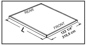
**Note:** Finished Slab dimensions, with lumber removed. Platform/Slab will extend 2" (5 cm) beyond floor frame on all four sides. Seal this 2" (5 cm) of wood with a roofing cement (not included), or bevel concrete when pouring for good water drainage.
