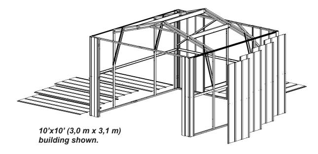
Working one side at a time, lift the **Panels** into place and secure top and bottom of **Panels** with **Small Screws**. Be sure to overlap ribs as shown on the previous page.
