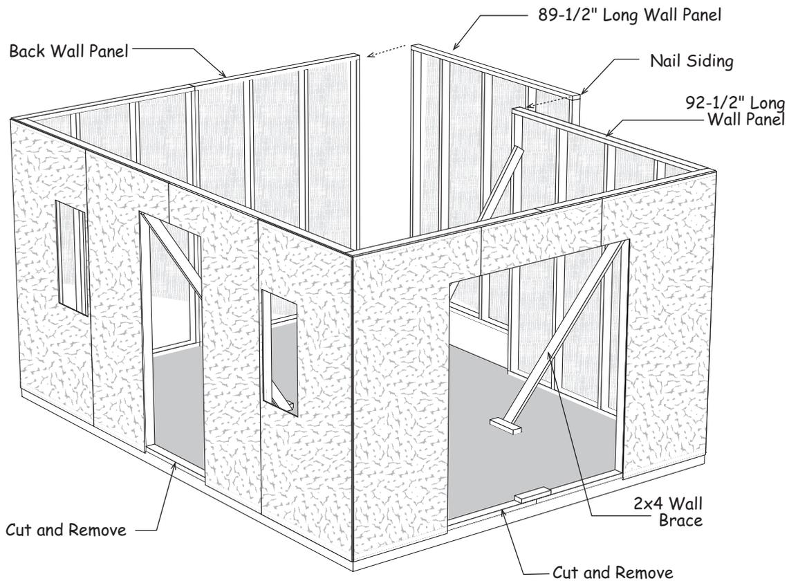
7. Cut and remove the bottom 2x4 in both door openings.
