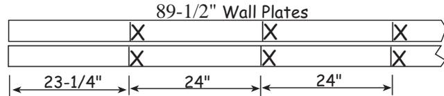
2. Install pre-cut wall studs between the top & bottom plates.
