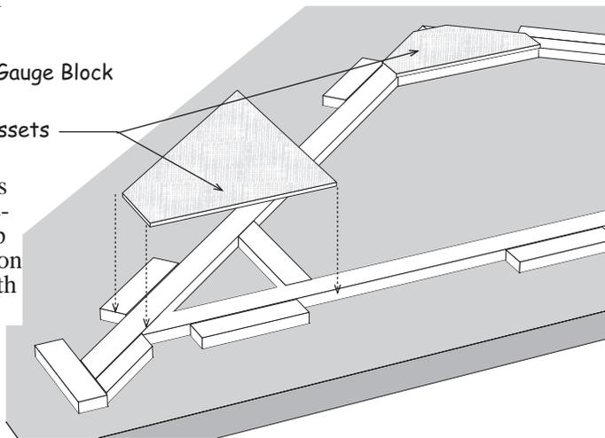
8. Repeat process to assemble (6) six more trusses. Do Not remove the 2x4 blocks around the perimeter of the truss until the gables are assembled in the next step.
