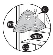
Fig.5: Use (S1) Screws. Fix (CB3XA) to (FCB) fitting.
