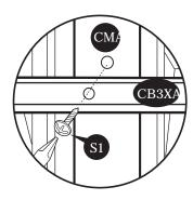
Fig.3: Use (S1) screws. Fix (CB3XA) to (CMA) columns.
