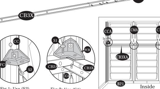
Fig.1: Use (S2) screws. Fix (FCB) fitting to (CCA). Leave it loose.
