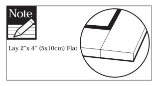
2. Using exterior grade CDX 3/4" (19mm) plywood, cut and fit together the sheets to form solid plywood floor as shown. Foundation must be square and level.
