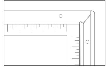
3. Attach each side panel (SP $\uparrow$ ) on top to the roof structure (RS1) and (RS3). Using a dia. 3mm (1/8") drill with a power drill, make two equal distance holes on the side panel through the roof structure. Drive a self tapping screw (S4) through the side panel to the roof structure. Repeat this for every side panel. See blowup.
