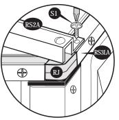
fig.3 Fix (RS2A) to 90 degree joint (RJ) through (RS3LA) & (RS3XA) with (S1) screw.
