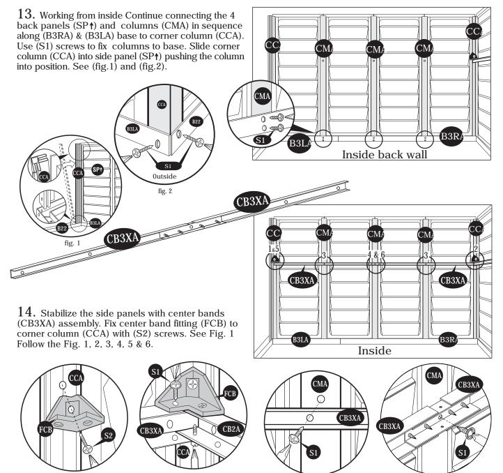
Fig.1: Use (S2) screws. Fix (FCB) fitting to (CCA). Leave it loose.
