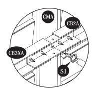
Fig.4: Fix to (CMA) with (S1) screw.
