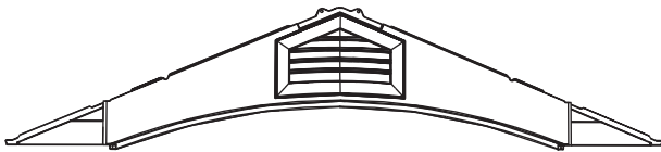
Entry Gable Assembly Front View
