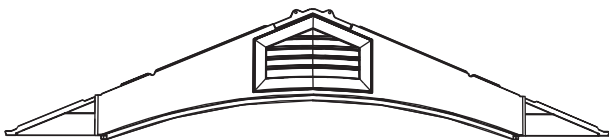
Entry Gable Assembly Front View
