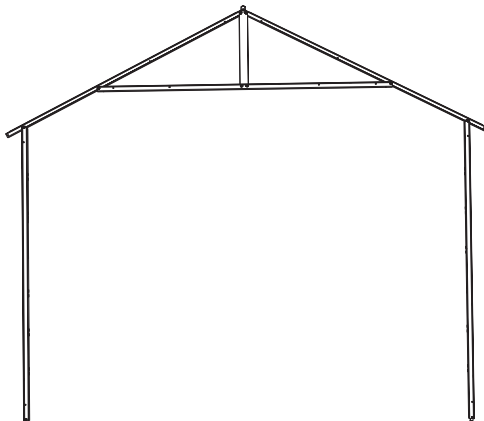
Truss Assembly (x1)
